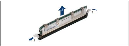
Figure 32: Removing a memory module
